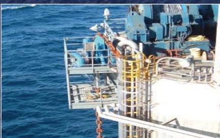
This compact chain jack has a holding capability of nearly twice that of adjacent mooring winches
